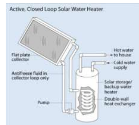
Figure 2-3: Active solar water heating system
